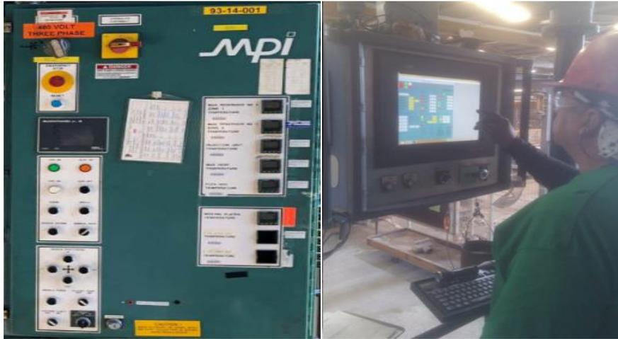
Control of a wax injector and a vacuum induction furnace.
